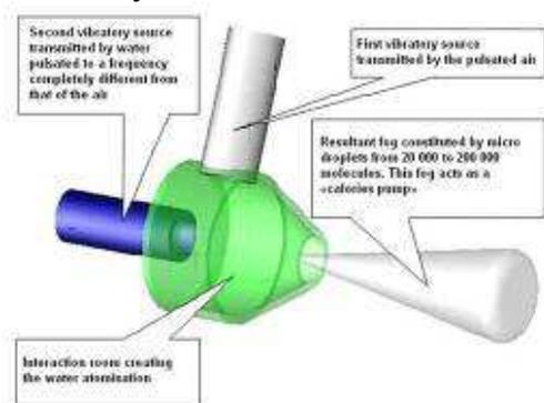
Figure 1 Schematic of atomizing reactor
